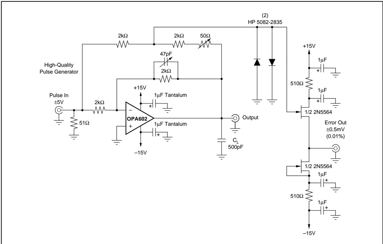
FIGURE 4. Settling Time and Slew Rate Test Circuit.
